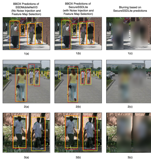
Figure 10. Comparison between SSD-MobileNetV3 (first column) and Secure SSDLite (ours, second column) bounding box predictions for samples from the PennFudan dataset. The yellow bounding boxes are the ground truth and the red boxes are the predicted boxes. The third column blurs the sensitive regions based on the predictions from the Secure SSDLite model with \alpha = 0.11 . Subfigures 1(a)–3(c) are examples of predicted bounding boxes with varying subjects and sizes.
