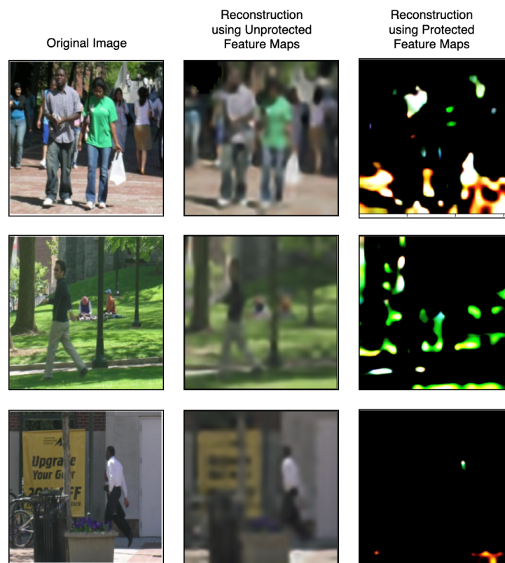
Figure 4. Comparison without our proposed scheme. The first column shows original images from the PennFudan dataset. The second column shows images reconstructed using unprotected feature maps (without our scheme), and the third column shows images reconstructed with an annulment factor of \lambda = 0.3 , noise variance of \sigma^2 = 0.4 , and mean of \mu = 0.1 . The annulment value used is based on a Gaussian distribution (i.e., k \sim \mathcal{N}(0, 1) ).
